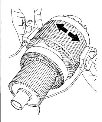
Checking armature for short to ground
